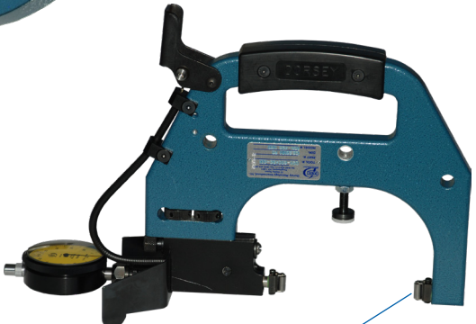
SDN Series frame shown with 2 wire floating rolls and thumb retraction
