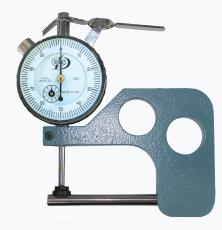
Part #FC2 Tube wall thickness
