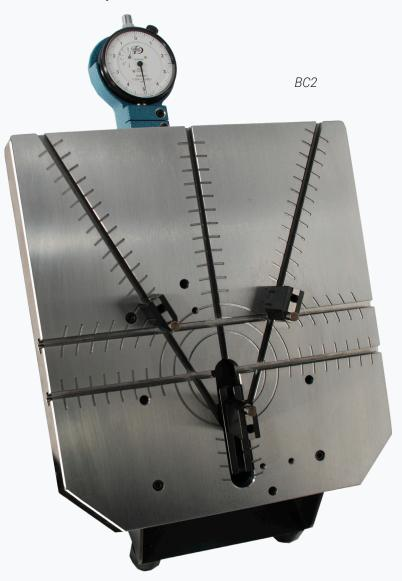
Note: Special ratio 4:5 dial indicator or electronically compensated digital indicator is recommended for 3 point non-diametric contact arrangement. See page 57 for optional indicators.
