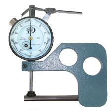
Part #FC2 Tube wall thickness
