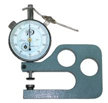
Part #FC1 1/2" dia. anvils,1" opening, 2" throat depth, with 2DM500-10F .001" Grad. dial with .5" travel
