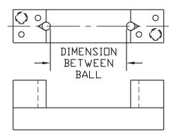
"V" Style pitch diameter setmaster, built per application
