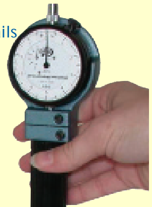
DBL-300 Shown being set with DBM- 1000 master
